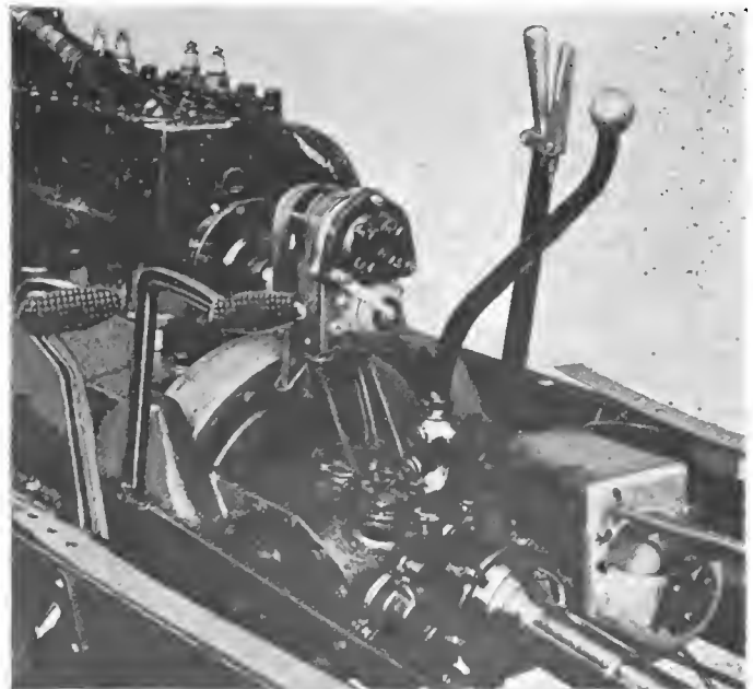
Mounting of magneto on bracket above gear case on new Briscoe, showing location of the combined starting motor and lighting generator
